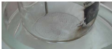
Figure SM 4.2.1.5.6: Consumption of I 2 solution becomes transparent (@ 70°C)
