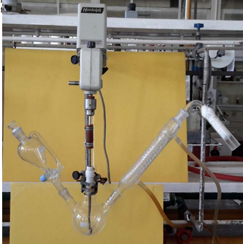
Figure SM 4.2.1.2.1 – Reaction set apparatus for triphenylmethanol
