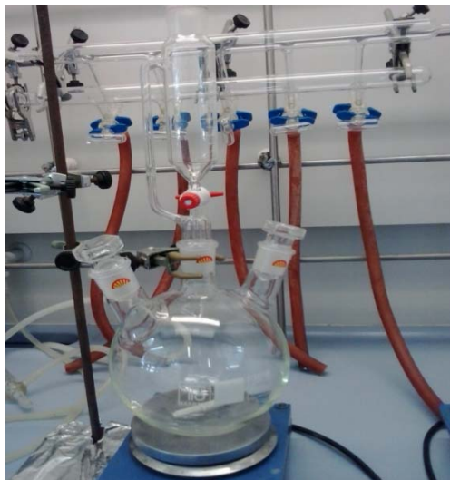
Figure SM 4.2.1.6.1. Three-necked round-bottom flask, equipped with addition funnel with pressure-equalization arm and with a magnetic stir bar.
