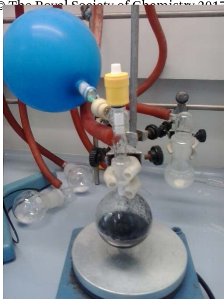
Figure SM 4.2.1.6.3. Round-bottom flask, equipped with a magnetic stir bar and a balloon with H 2 (Hydrogenation step)
