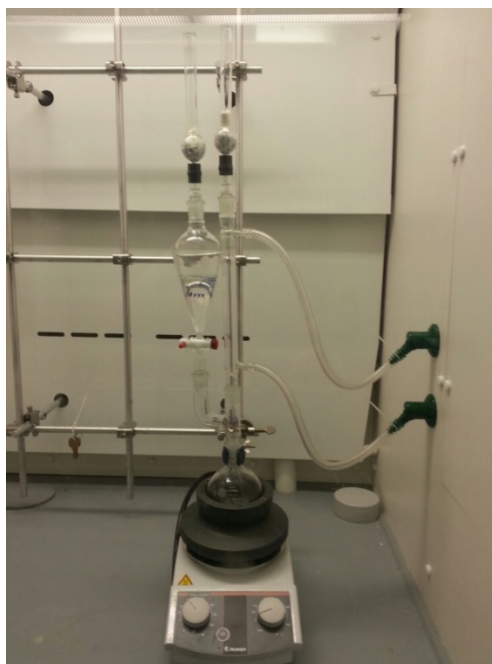
Figure SM 4.2.1.1.1: Grignard reaction dropwise addition apparatus
