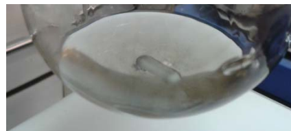
Figure SM 4.2.1.5.7: Almost entire consumption of Mg. The PhMgBr produced is ready to be used.
