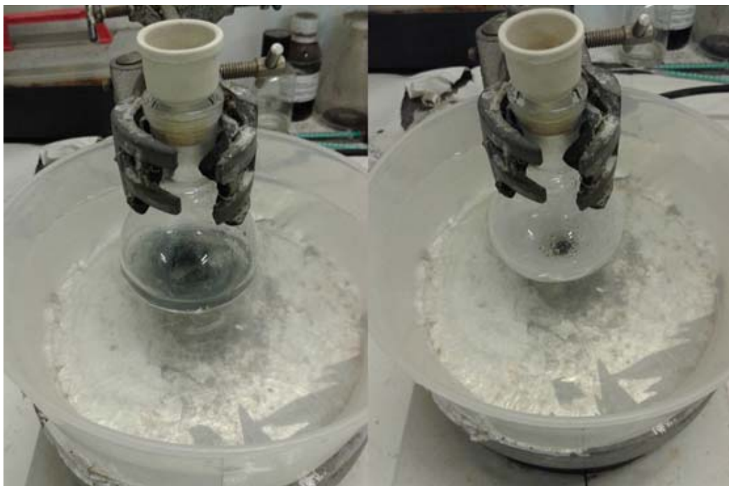
Figure SM 4.2.1.3.4: Reaction apparatus before addition of allyl bromide (left, grey appearance) and 10 minutes after addition of allyl bromide (right, white appearance).
